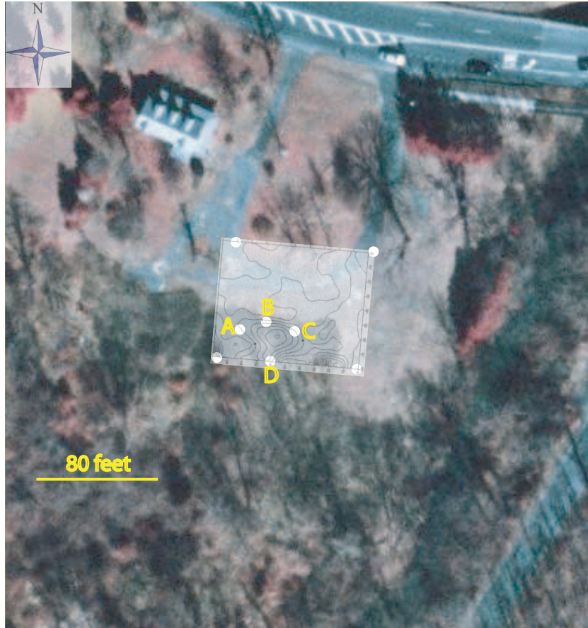
Figure 1: Tinton Manor Iron Works with Elerctomagnetic contour map overlaying air photo of investigation area
